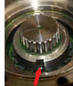
4. Push locking tabs down using a screwdriver
