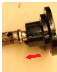
7. Push shaft out in the direction indicated by the arrow
