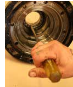
7. Tap out bearing and shaft seal using a screwdriver and hammer
