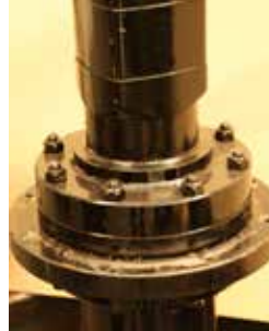
2. Remove motor bolts & remove motor
