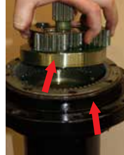
3. Remove gear set & ring gear
