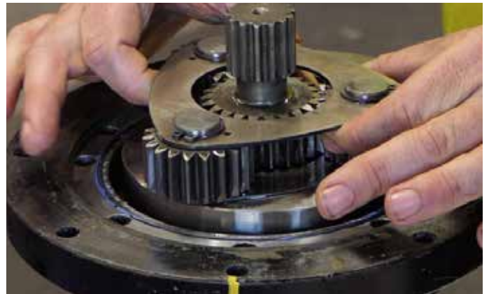
24. Replace the gearset. Skip step for PDD.
