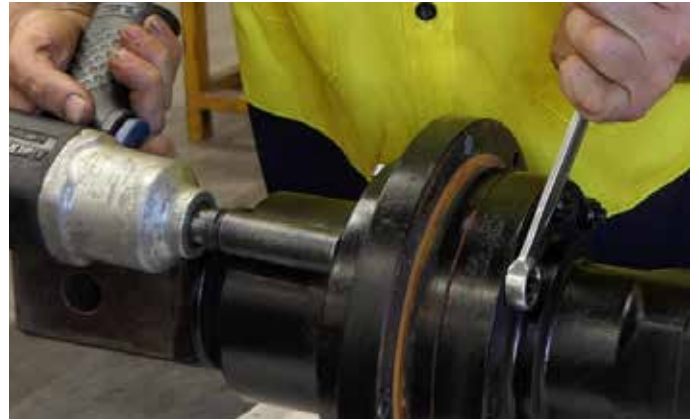
6. Remove the motor bolts and the motor with a 16mm socket or spanner and 17mm on the opposite side. Skip step for PDD.
