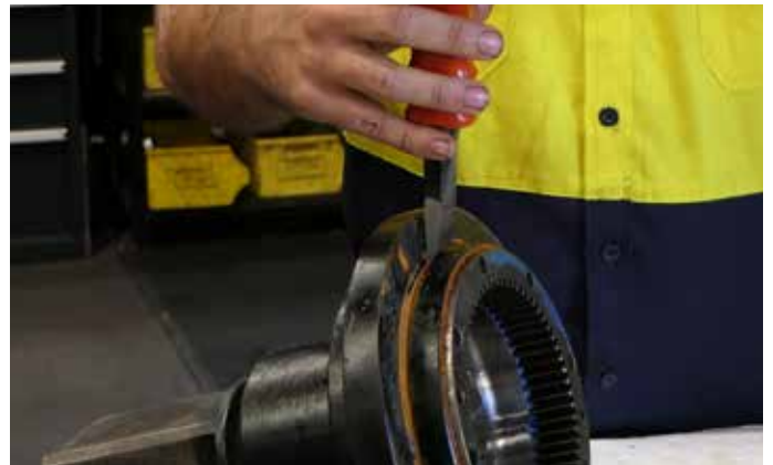
8. Remove the ring gear. A hammer and chisel may be necessary. Skip this step for PDD.
