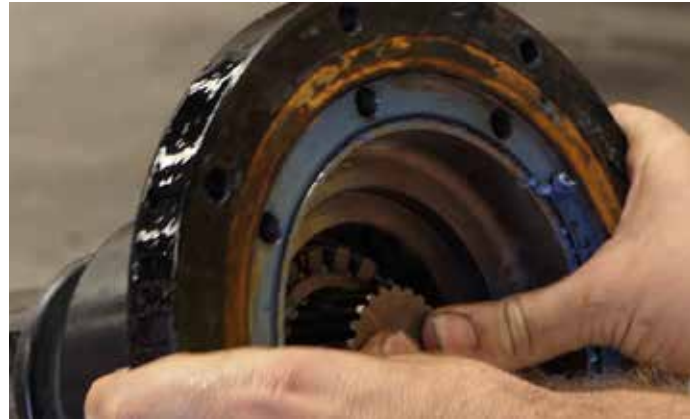
10. Push the shaft out and remove the tab washer.
