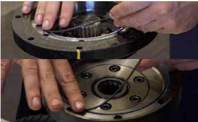
23. Place the new O-rings in gearbox and motor (optional use of blue gasket sealer). PDD units only require the motor O-ring.
