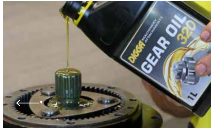
26. Fill with oil to 5mm below the top of the ring gear* (PDD: below the lip) and allow time for it to settle to the bottom. For ease of assembly, clamp shaft with a vice or similar.
