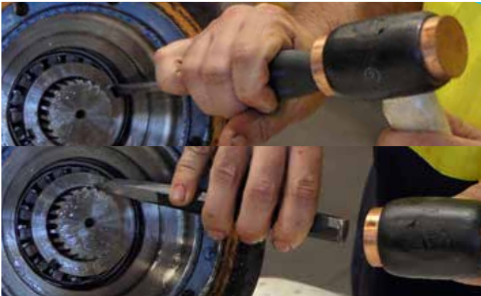
9. Push the locking tab down & unscrew the lock nut using a chisel and hammer.
