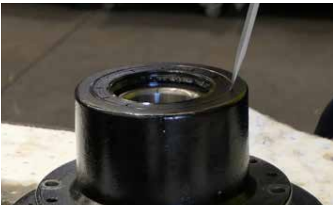
11. Tap out the shaft seal using a screwdriver and hammer. Remove the bearing. Do not hit outer roller as it may cause bearing damage.
