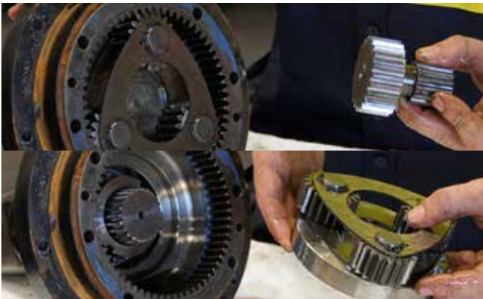
7. Remove the gearset. Skip this step for PDD.
