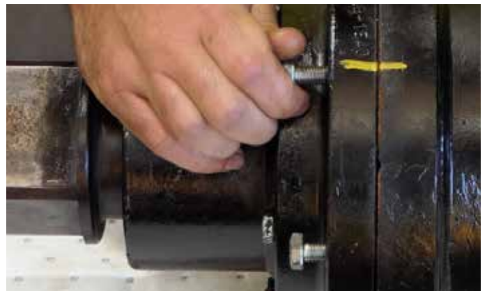
28. Guide hoses through the hood to replace the hood and replace hood bolts (torque: 55Nm) lining up previously marked alignment lines. PDD: Replace hood and hood bolts.
