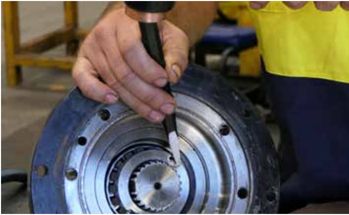
21. Screw the nut into place with flat side up to approx 170Nm. With a chisel & hammer, turn nut recess so it lines up with locking tabs.
