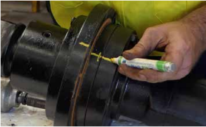
5. Continue the alignment mark to match the previous mark at the center of the motor.
