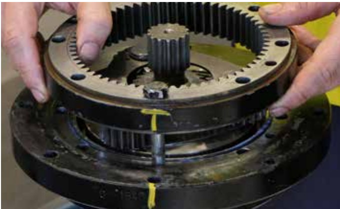
25. Replace the ring gear by using a bolt to help guide it into place. Skip step for PDD.
