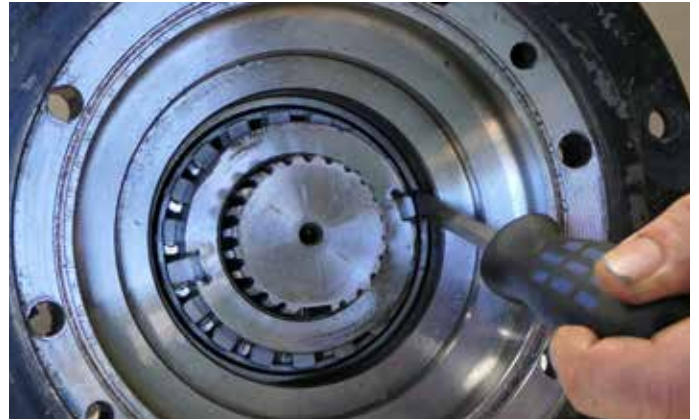
22. Lock the nut and bend the tab washer tabs into the recess of the nut.
