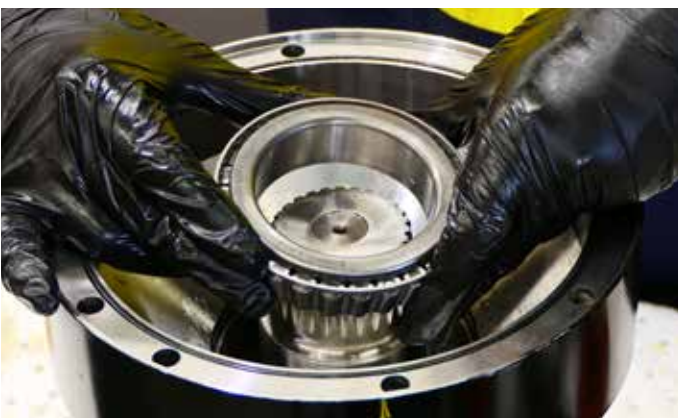
19. Turn the housing over and stand it on the shaft. Reinsert the upper bearing.
