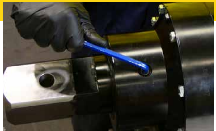
2. Using an 8mm Allen key, remove the bung.
