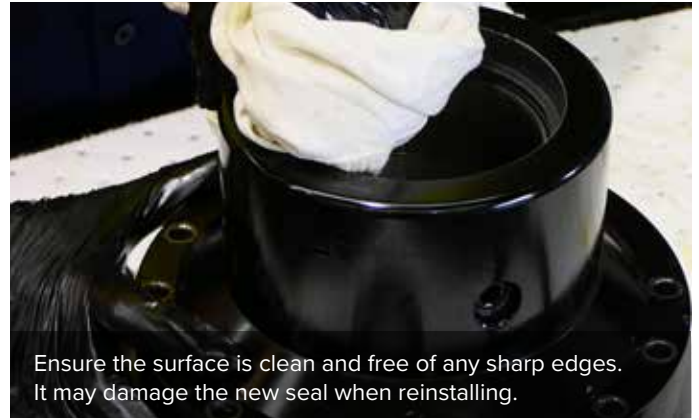
14. After the shaft seal has been removed, clean and inspect the parts. Return the lower bearing inside the housing.
