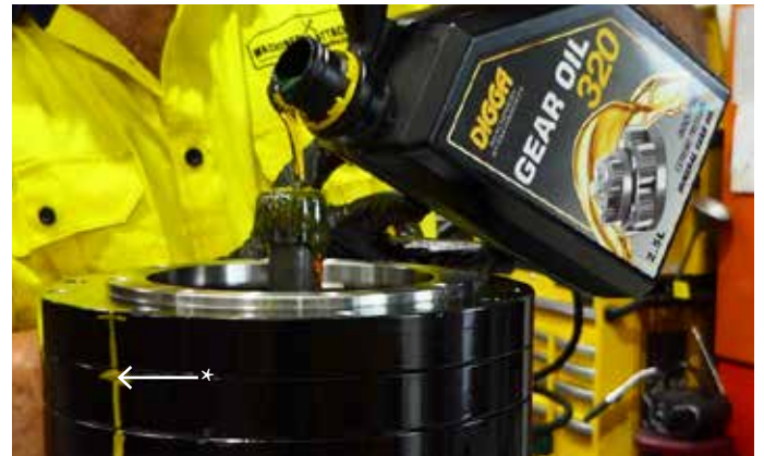
26. Fill with oil to 5mm below the top of the ring gear*, and allow time for it to settle to the bottom. For ease of assembly, clamp shaft with a vice or similar.
