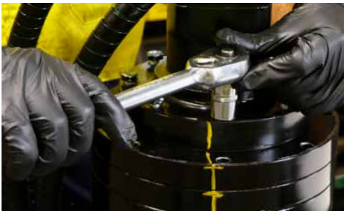
27. Replace the motor and motor bolts lining up previously marked alignment lines (optional: Loctite 243 Thread locker - medium strength on bolts).
