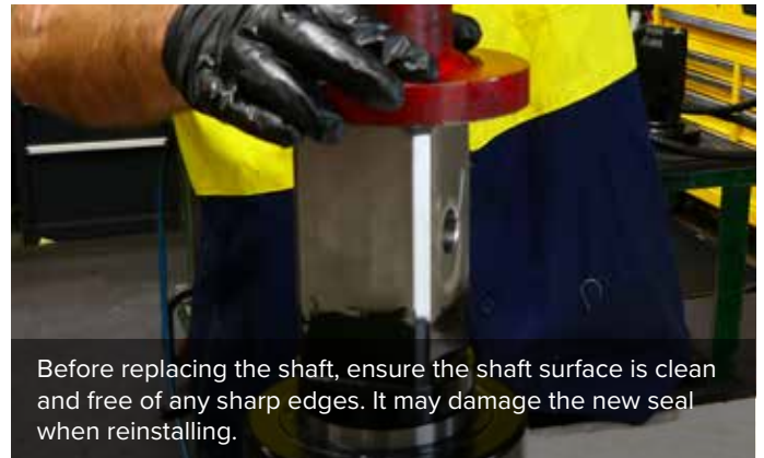
18. Using a flat metal plate and hammer, tap the shaft back into the housing, until the shaft is fully inserted.
