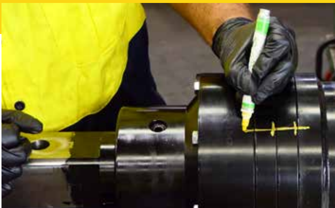
1. Lay the drive unit on the ground with the oil bung fill facing up. Mark a line on the hood & gearbox lining up with the center point of the hoses.
