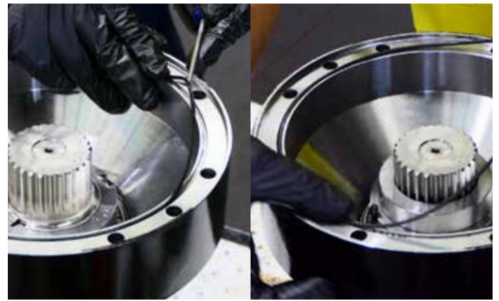
22. Remove the old O-rings from the input housing and ring gear. Clean both surfaces with a clean rag. Insert the new O-rings into the input housing and ring gear.
