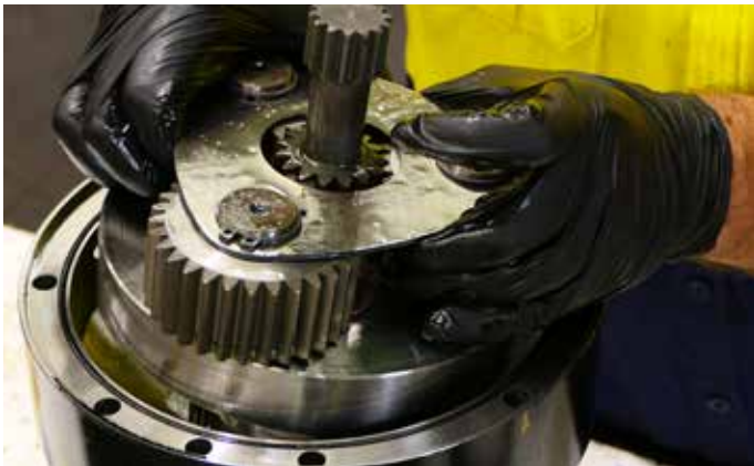
23. Re-insert the shaft spacer and ensure the flat side points towards the gearset. Replace the gearset.
