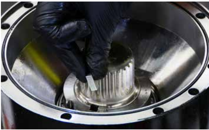
21. Insert the key and turn nut recess to make sure the shaft recess and lock nut recess no longer line up. This will secure the key (a chisel & hammer can be used).
