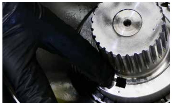
20. Screw the lock nut into place with flat side up. Do this whilst turning the housing until the bearing begins to feel firm. This will also line up the shaft key-way.
