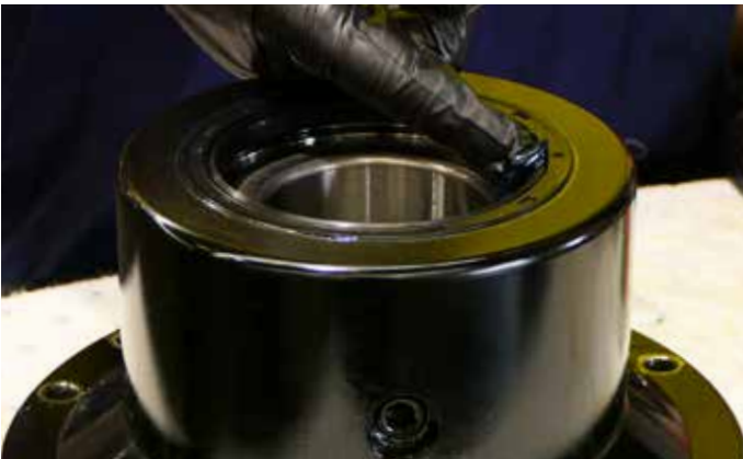
17. Apply grease to the inside of shaft seal. Note: For PD4HF-PD10HD & PD12, you will then need to reinstall the seal protector.
