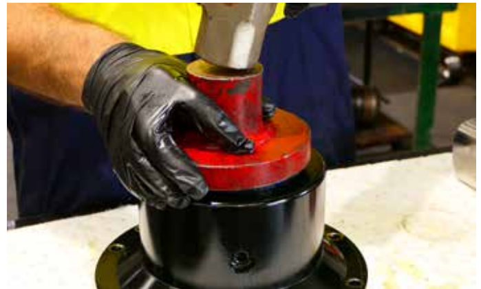
16. Place the shaft seal in position ensuring it is level & tap it in with a flat metal plate and hammer, so it sets evenly.
