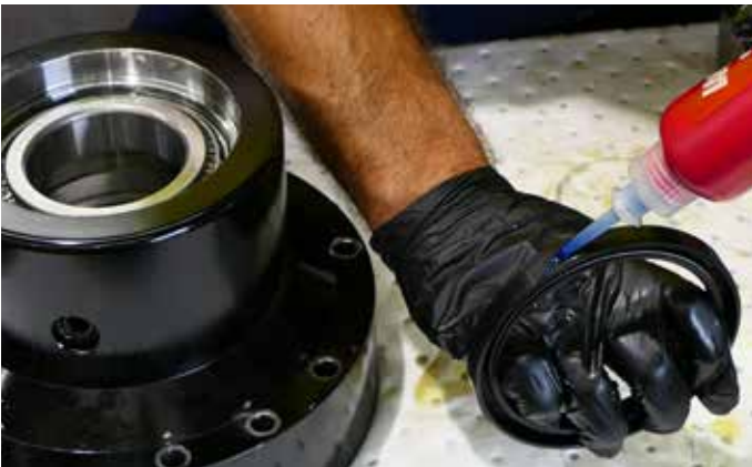
15. Apply Loctite (243 Thread locker, medium strength) around the outside of the shaft seal.
