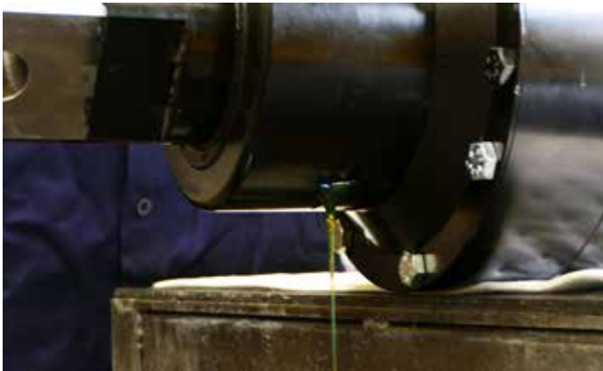
3. Rotate the unit until the oil fill hole is facing the ground and drain the oil. Apply Loctite 567 thread sealant to the oil bung, and reinsert, after the oil has completely drained.
