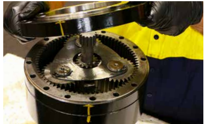
24. Replace the ring gear, and for PD6-PD10, the input housing, lining up the previously made marks.
