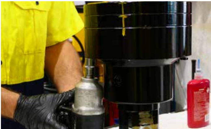
25. (PD6 / PD7 only) Insert the 2 longer bolts into the unevenly spaced holes on the gearbox housing (Use medium strength 243 thread locker). Secure the top-most ring above ring gear.
