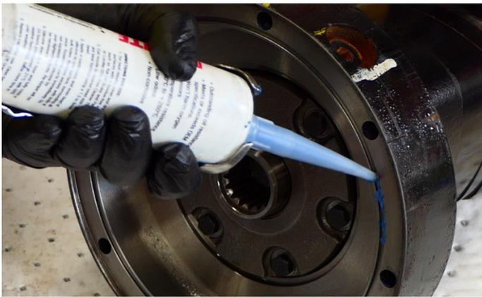
45. Apply a light bead of oil-resistant sealant (Flange sealant – Loctite – SI 587) into the O-ring gauge of the Motor
