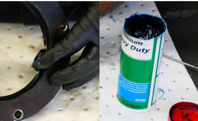
25. Apply grease to the inside of the shaft seal.
