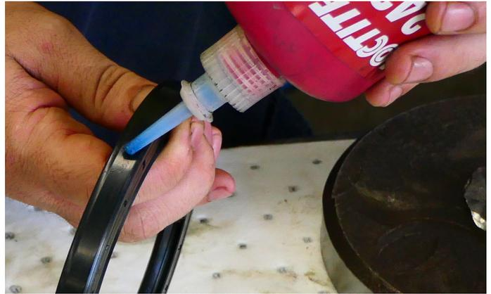
22. Before reinstalling the seal, use an alcohol-based cleaner on the seal protector surface (important). Apply Loctite (243 thread locker, medium strength) around the outside of the shaft seal.
