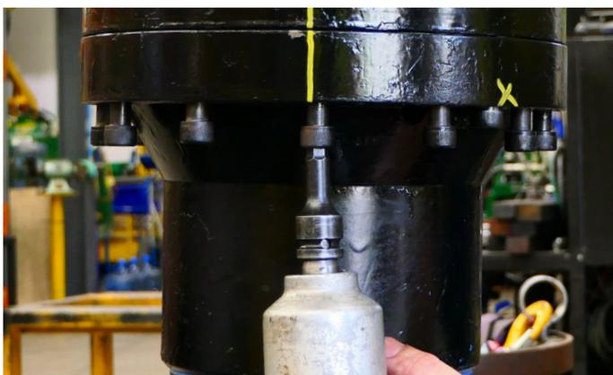
51. Fasten the hood bolts - Use Loctite 243 medium strength thread locker. Torque to 184Nm.
