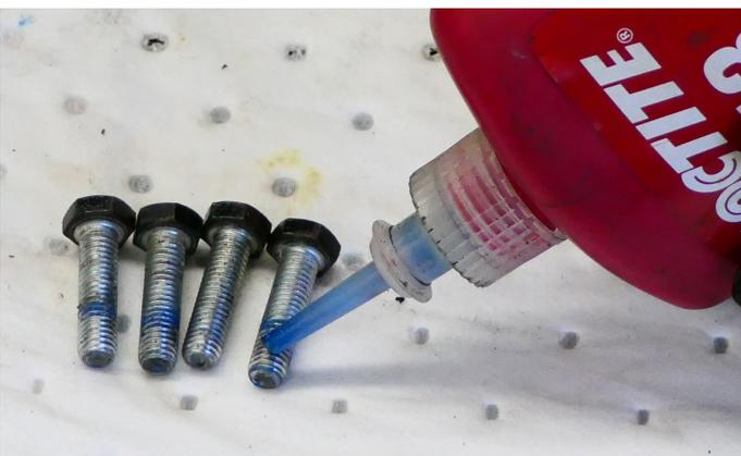
27. Apply Loctite 243 thread locker, medium strength to the seal protector bolts.
