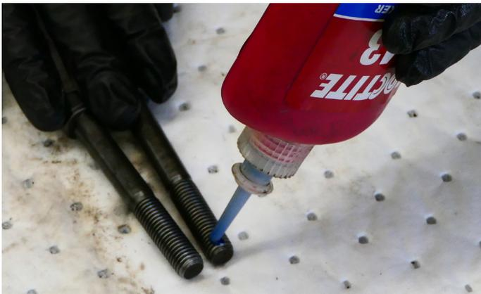
39. Loctite 243 thread locker, medium strength may be used on bolts which hold the hood spacers to the gerset housing.
