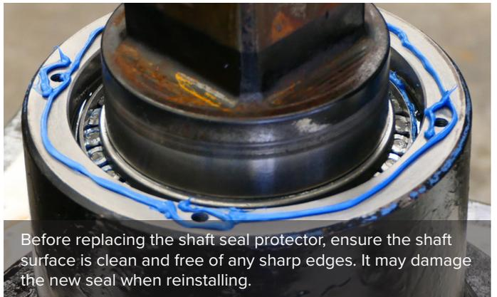
Before replacing the shaft seal protector, ensure the shaft surface is clean and free of any sharp edges. It may damage the new seal when reinstalling.
