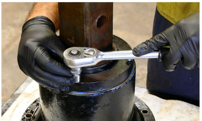
28. Replace the shaft seal protector by fastening the bolts with a 13mm socket or spanner.
