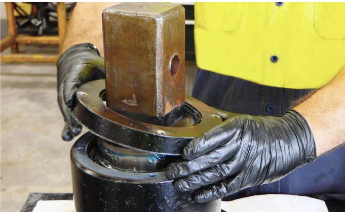
17. Remove the seal protector. You may require a copper hammer to break the seal.
