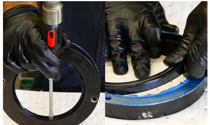
18. With a screwdriver & hammer, remove the seal from inside the seal protector.
