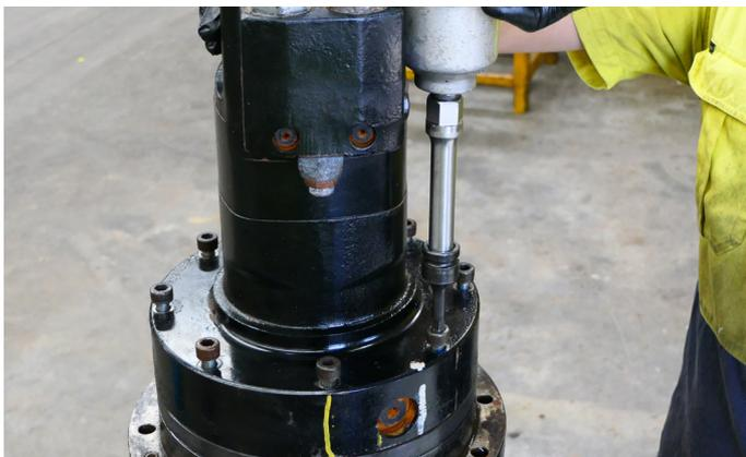
49. Fasten motor bolts. Use Loctite 243 Thread locker - medium strength on bolts.
