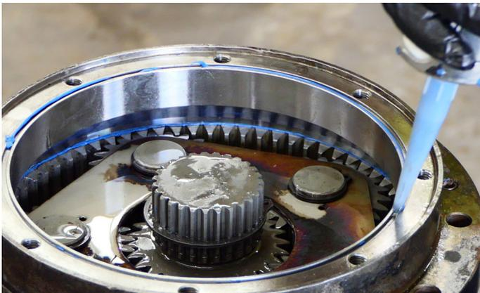
41. Apply a light bead of oil-resistant sealant (Flange sealant – Loctite – SI 587) into the O-ring gauge of the interim housing.
