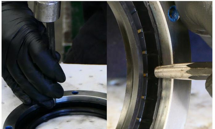
24. With a pin punch & hammer, Tap the shaft seal into the seal protector (only hitting the outside wall of the shaft seal).
