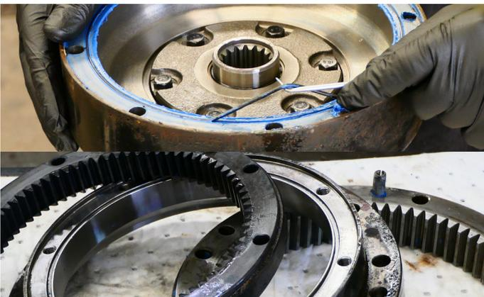
19. Remove all (4) old O-rings on input housing (motor), output housing, interim housing and ring gear.
