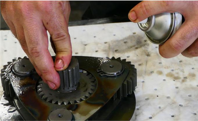
21. Clean down all parts. We recommend using degreaser / alcohol-based cleaner to remove old oil.
