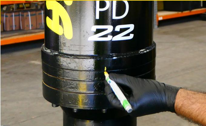
1. Place the drive unit on a stand. Alternatively, with an auger attached, drill a hole into soil, and leave the auger in as a stand. Mark a line on the hood and gearbox between the hoses.
