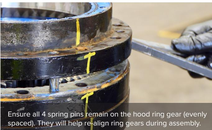
Ensure all 4 spring pins remain on the hood ring gear (evenly spaced). They will help re-align ring gears during assembly.
