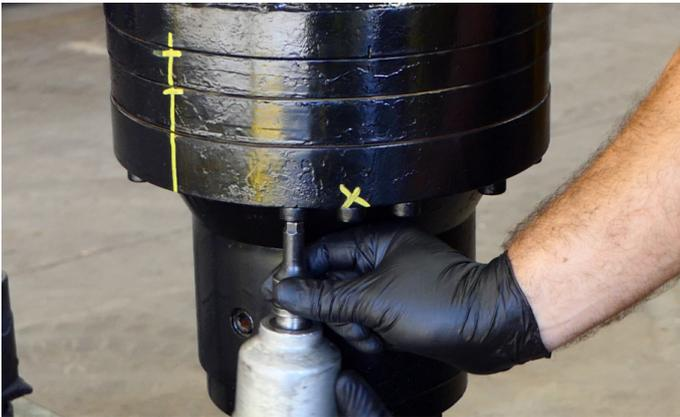
3. Remove the hood bolts with a 10mm socket (allen key) and remove the hood.
