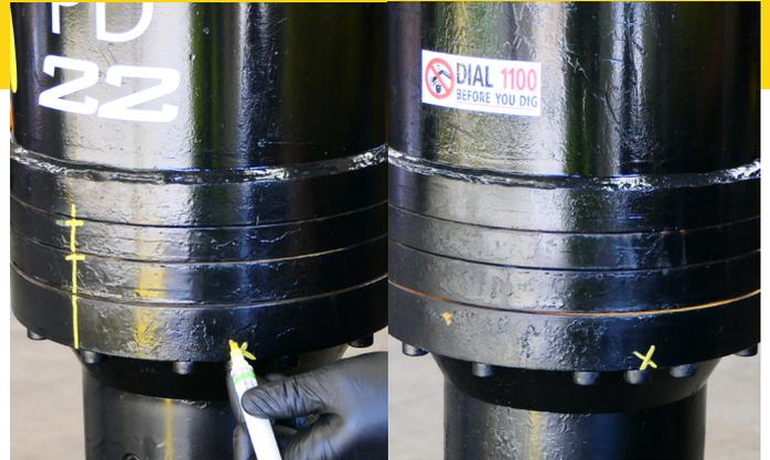
2. Mark the 2 bolts which fasten the hood spacers to the gearset housing (located opposite each other, between 3 evenly spaced bolts).
