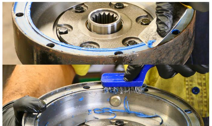
20. Clean all parts with a scraper & scourer or steel brush to remove excess sealant and contaminants. We advise using an air gun or air tool to ensure no contaminants are left inside the housing.
