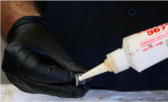
29. Apply Loctite 567 thread sealant to the oil bung.
