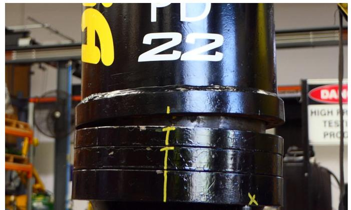
50. Replace the hood. Align the previously marked line with those marked on the housing.
