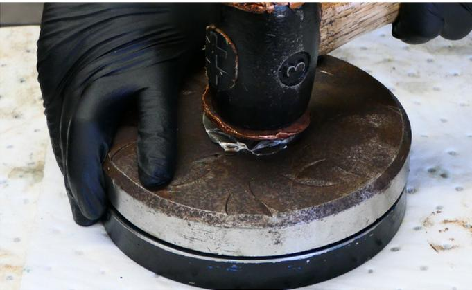
23. Position the shaft seal level, with the open side facing up. Tap it in evenly using a flat metal plate & hammer.
