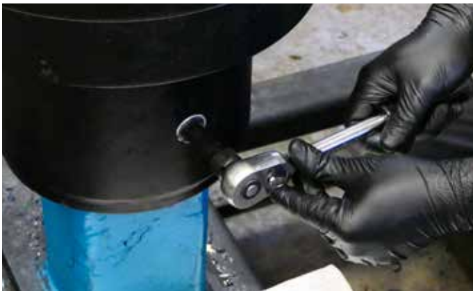
7. Once the motor has been removed, use an 8mm Allen key to remove the oil bung. Let the oil drain.
