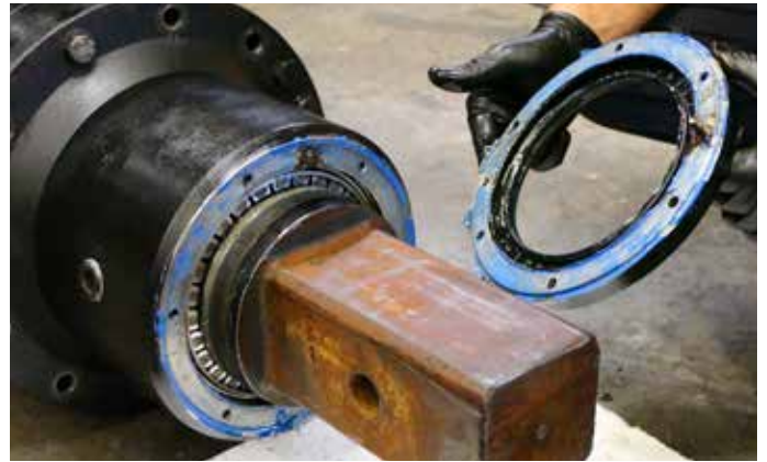
16. Remove the seal protector. You may require a copper hammer to break the seal.
