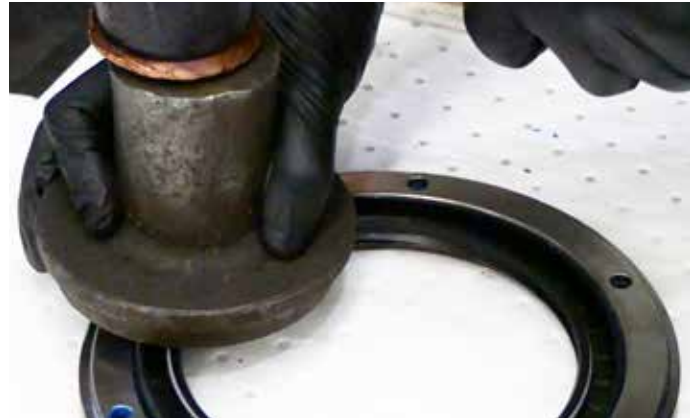
22. Position the shaft seal level, with the open side facing up Tap it in evenly using a flat metal plate & hammer.
