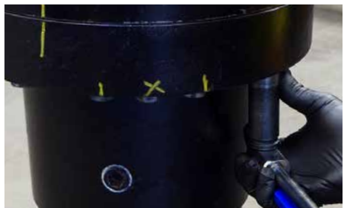
52. Fasten the hood bolts with a 13/16 socket or spanner. Torque to 147Nm.
