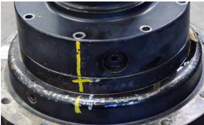
47. Replace the motor lining up previously marked alignment lines.
