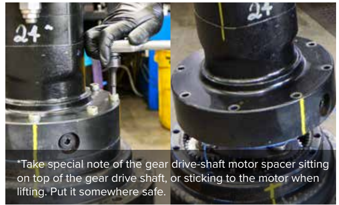
6. Remove the motor bolts and motor with a 10mm socket (allen key). If using a rattle gun we recommend using an extension bar.
