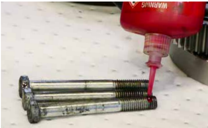
37. Loctite 263 thread locker (high strength) may be used on bolts which hold the hood spacers to the gearset housing.
