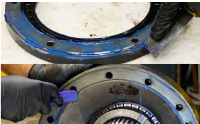
19. Clean all parts by using a scraper & scourer or steel brush to remove sealant / contaminants. We recommend using an air gun / air tool to ensure no dirt is left inside the housing.
