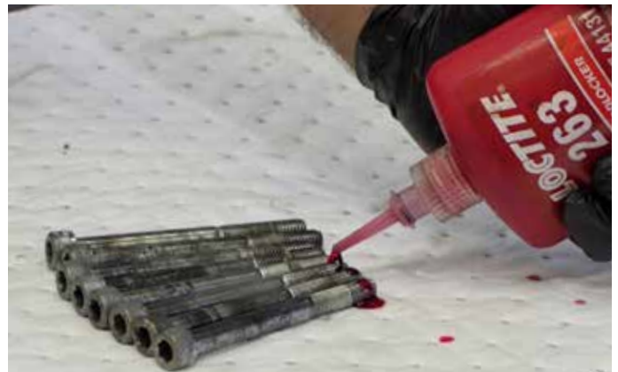
48. Use Loctite 263 Thread locker - high strength on the bolts.
