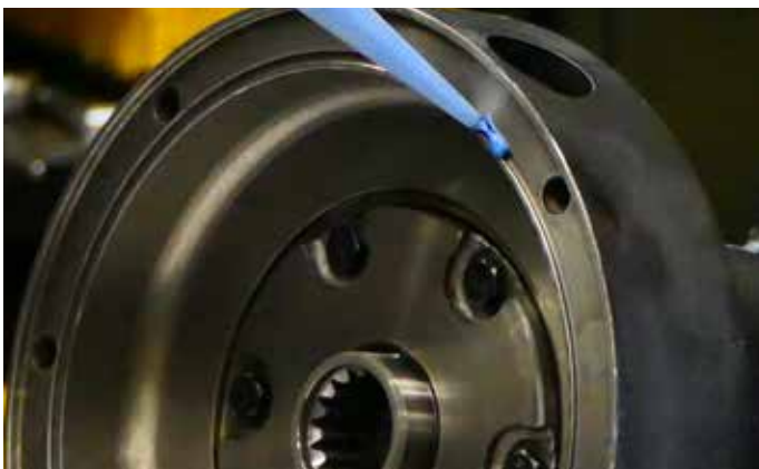
43. Apply a light bead of oil-resistant sealant (Flange sealant – Loctite – SI 587) into the O-ring gauge of the Motor
