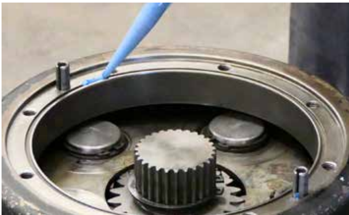
39. Apply a light bead of oil-resistant sealant (Flange sealant – Loctite – SI 587) into the O-ring gauge of the interim housing.
