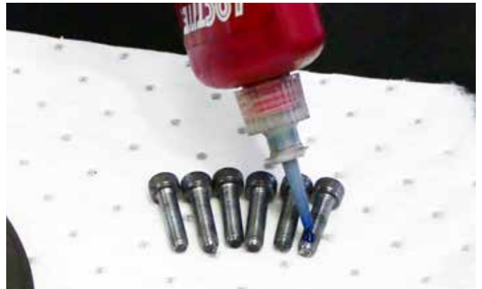
26. Apply Loctite 243 thread locker, medium strength to the seal protector bolts.
