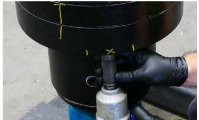
38. Fasten the hood spacers to the gearset housing by replacing the 2 bolts at the marking points, with a socket or spanner. Torque to 147Nm
