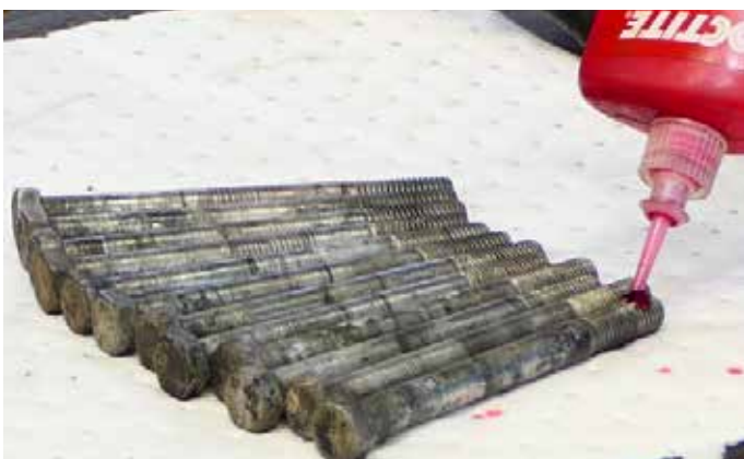
51. Use Loctite 263 high strength thread locker on the hood bolts.
