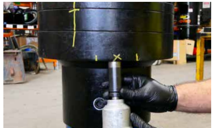
10. Unfasten the last 2 bolts from the gearset assembly housing to release the interim housing and ring gear.
