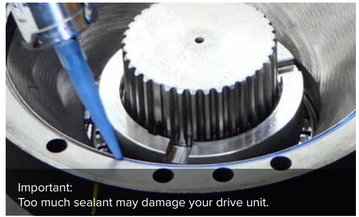
30. Place the output housing (with shaft) back on the stand. Apply a light bead of oil-resistant flange sealant (Loctite SI 587) into the O-ring gauge.
