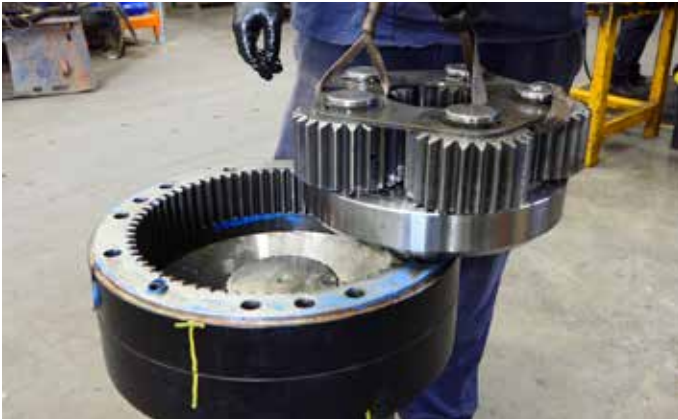
13. Remove the gear set. Lifting equipment will be required.
