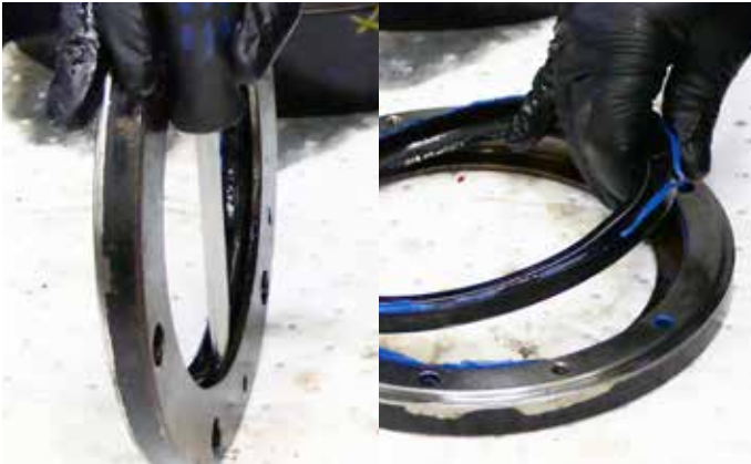
17. With a screwdriver & hammer, remove the seal from inside the seal protector ensuring you do not damage the housing.
