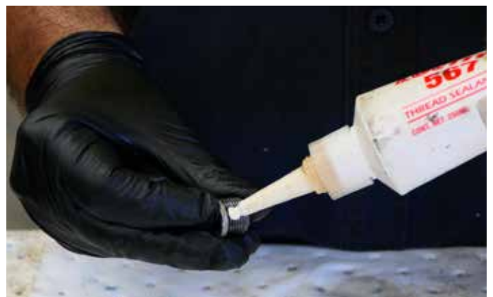
28. Apply Loctite 567 thread sealant to the oil bung.
