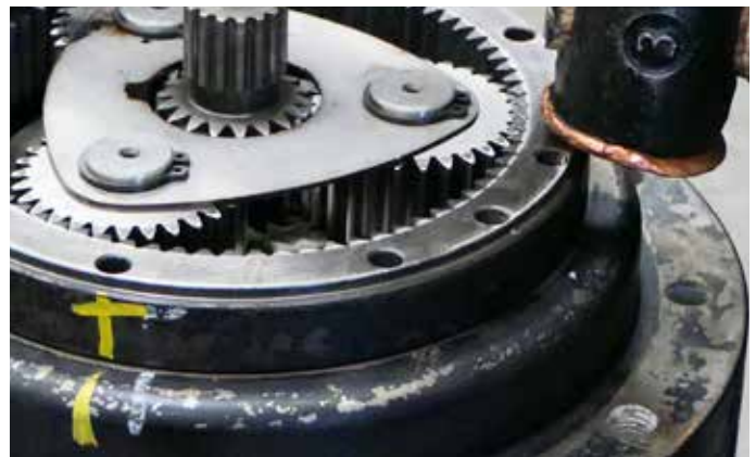
42. Replace ring gear - Line up previously made marks. Tap down ring gear with a copper hammer as needed. Use the hammer to ensure housing and spring pins are fully inserted.
