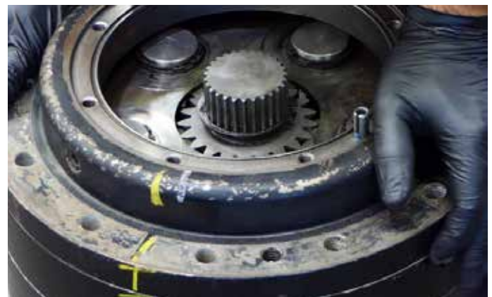
36. Place interim housing on the ring gear.
