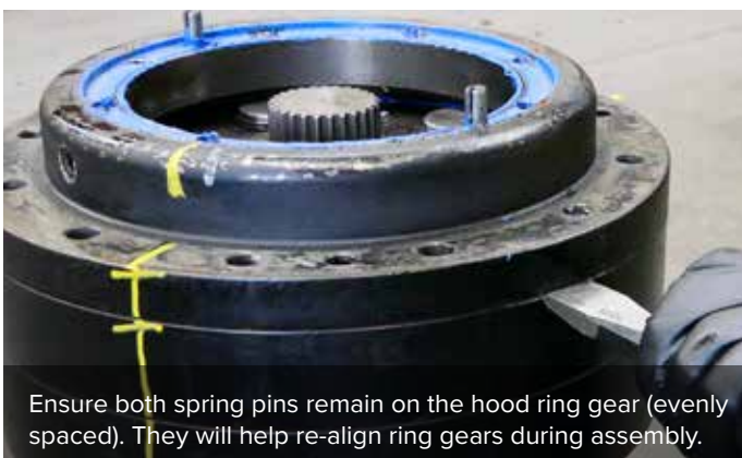
11. Using a chisel & hammer, remove the interim housing. A pry bar may be required.
