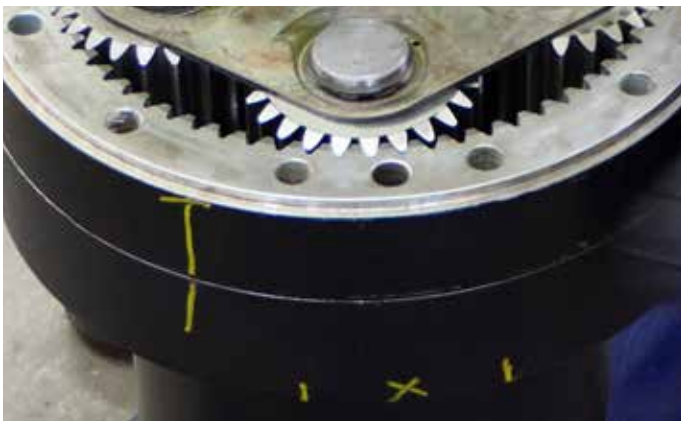
33. Replace the ring-gear. Ensure parts are aligned correctly with previously drawn alignment marks.
