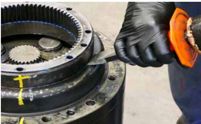
9. Remove the ring gear. Use a chisel and hammer to loosen it.
