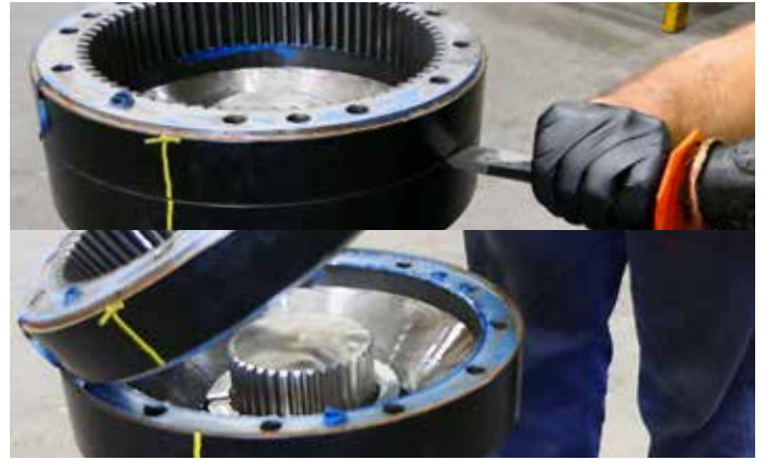
14. Using a chisel & hammer, remove the hood ring gear.
