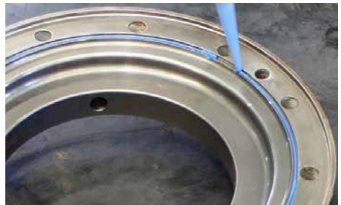
34. Apply a light bead of oil-resistant sealant (Flange sealant – Loctite – SI 587) into the O-ring gauge of the interim housing.
