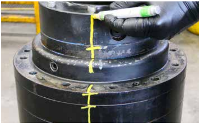
5. Continue the alignment mark to match the previous mark at the centre of the motor.
