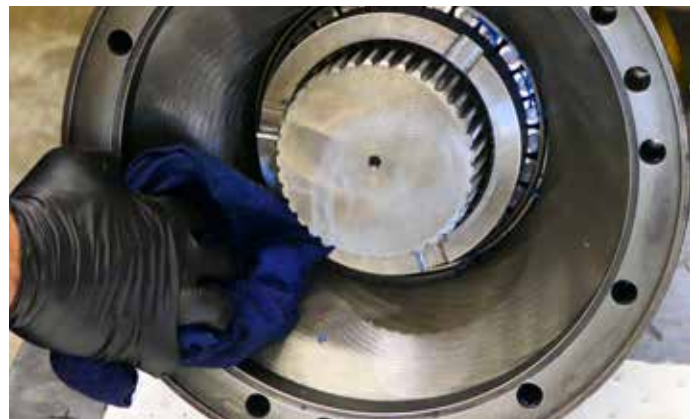
20. Thoroughly clean down all parts. We recommend using degreaser / alcohol- based cleaner to remove old oil.
