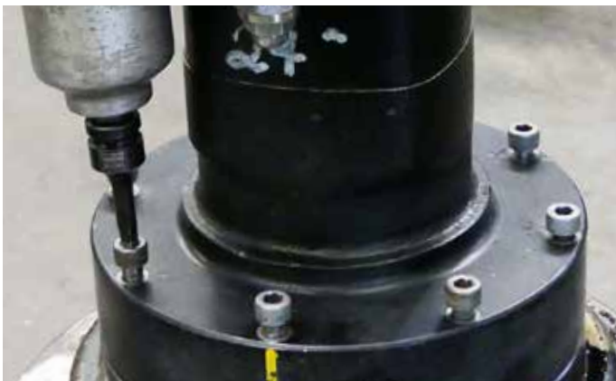
49. Fasten the motor bolts. Torque to 95Nm.
