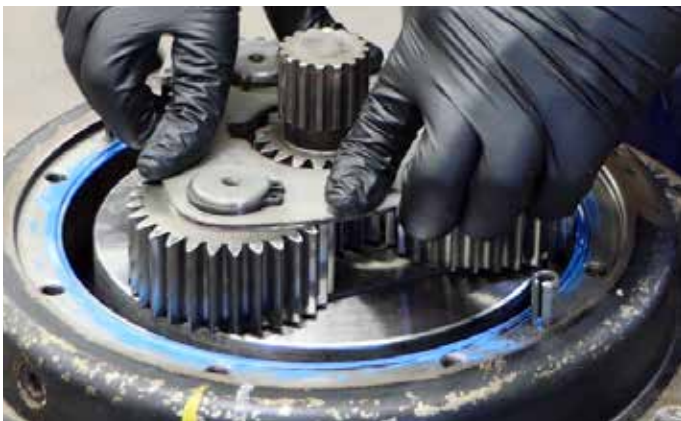
41. Replace the gearset. A soft copper hammer may be used to secure gearset in place.
