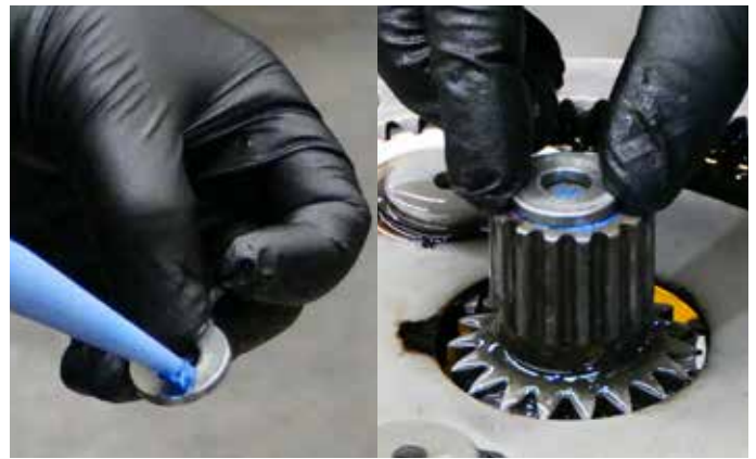
46. Apply a light bead of oil-resistant sealant (Flange sealant – Loctite – SI 587) to the drive shaft spacer. Secure it in place (between the motor and gear drive shaft).
