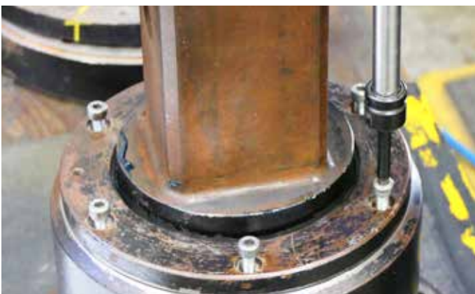
27. Replace the shaft seal protector by fastening the 8mm socket cap screws with a 6mm allen key socket or allen key.
