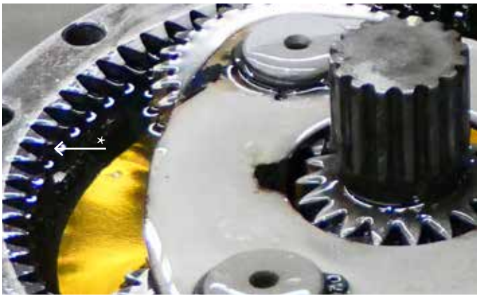
45. *Fill to 5mm below the top of the ring gear. Allow time for the oil to settle to the bottom.
