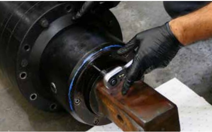
15. Place the housing on a flat surface with the shaft facing up. Remove the seal protector by using a 6mm allen key socket or allen key, to remove the 8mm socket cap screws.
