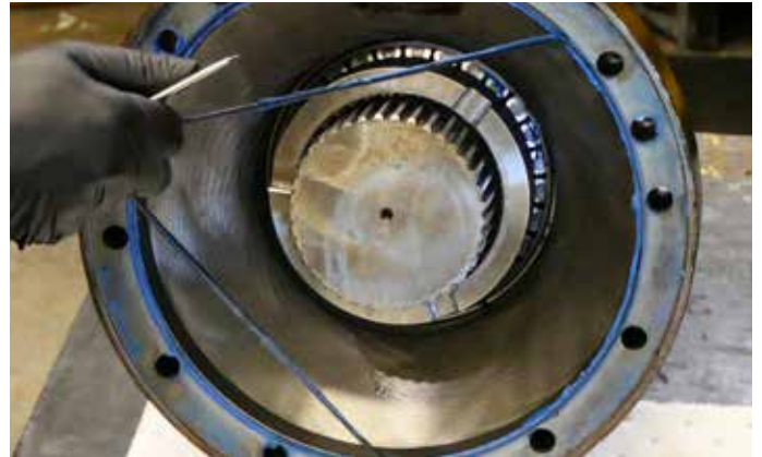
18. Remove all (4) O-rings on input housing (motor), output housing, interim housing and ring gear.
