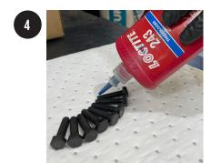
APPLY LOCTITE TO NEW BOLTS. DO NOT USE THE OLD BOLTS.
