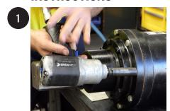
UNDO BOLTS HOLDING THE HOOD TO THE GEAR BOX
