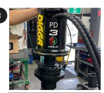
THREAD THE HOSES THROUGH THE HOOD OPENING AND LOWER THE NEW HOOD ONTO GEAR BOX
