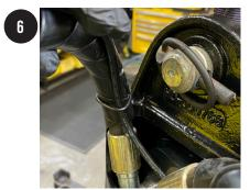
THREAD THE O-RING OVER ONE OF THE HOSES AND INSERT THE HALO LEAD IN CABLE UNDER IT
